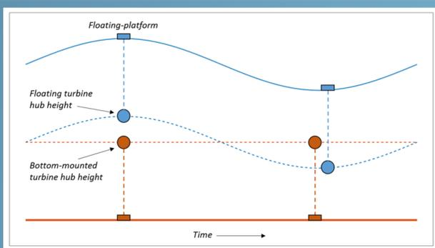
Schematic showing different configurations of floating-platform (blue) and bottom-mounted (red) turbines in the water column.
