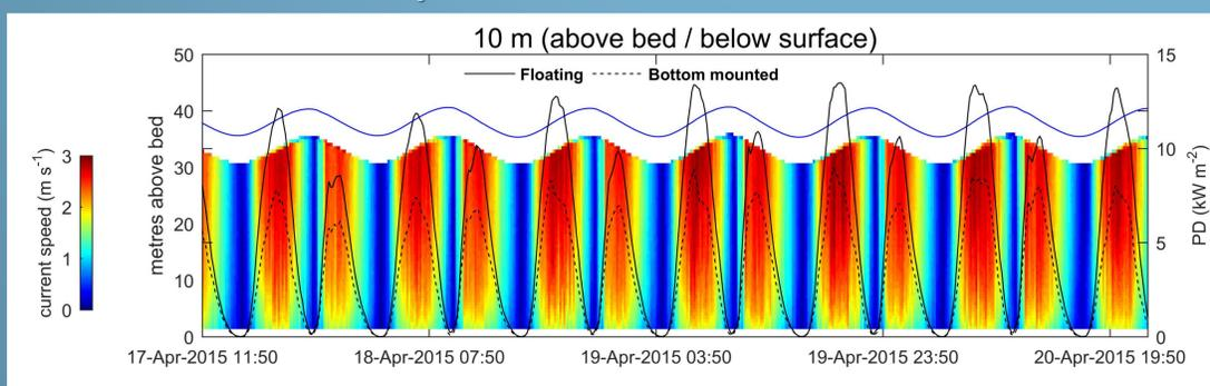
Time series of observed tidal current speeds and elevations during spring tides at the ADCP location – with calculations for Power Density from fixed vs floating tidal stream devices, at 10 m above bed / below surface
